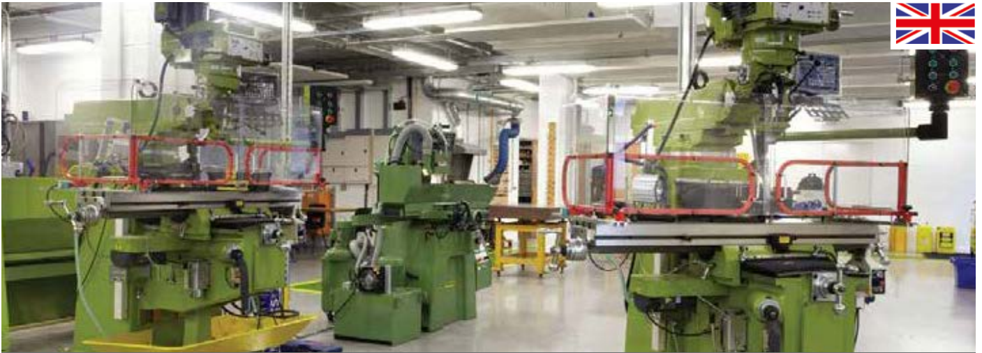
Design & Technology workshop installation, equipment and supplies by Technology Supplies Ltd WM40 Turret Mill - Toolroom quality, high precision mill with WMT Hydraulic Surface Grinder in background
